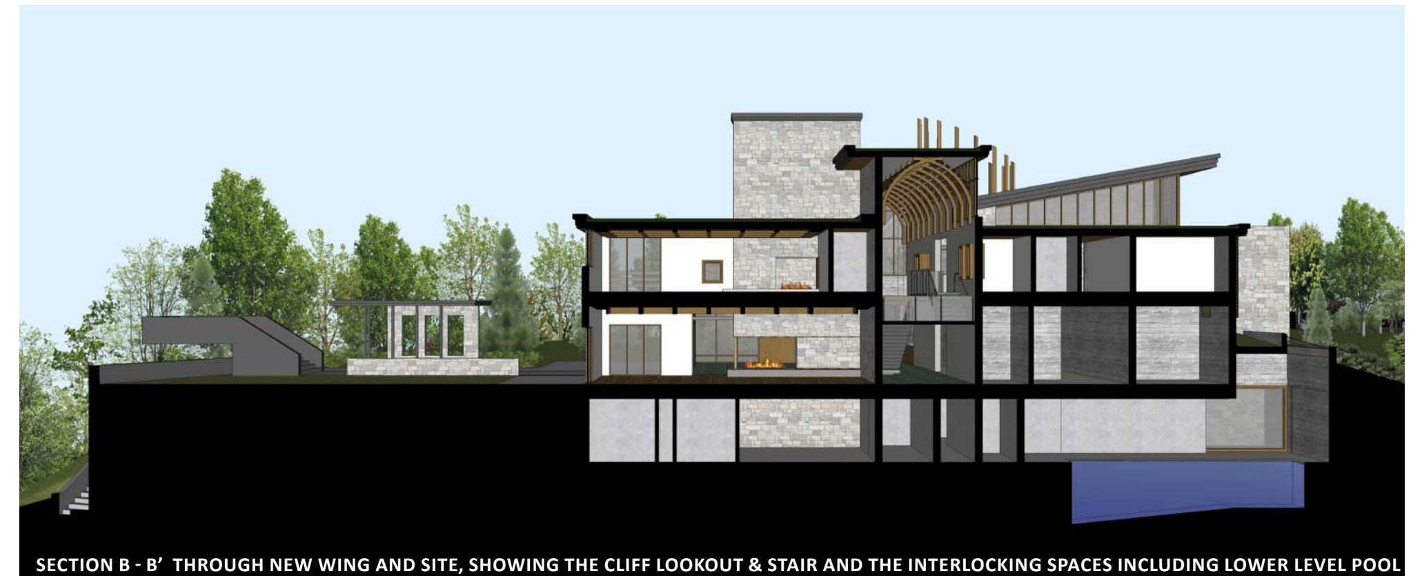
SECTION B - B' THROUGH NEW WING AND SITE, SHOWING THE CLIFF LOOKOUT & STAIR AND THE INTERLOCKING SPACES INCLUDING LOWER LEVEL POOL
