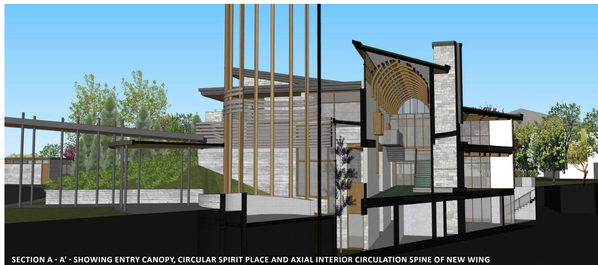
SECTION A - A' - SHOWING ENTRY CANOPY, CIRCULAR SPIRIT PLACE AND AXIAL INTERIOR CIRCULATION SPINE OF NEW WING
